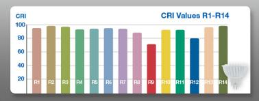
THE CRISP SERIES MR16 7.5W lamp features a typical CRI 92, R9 70 and R13 96, providing crisp and vibrant colors across the whole spectrum. Its exceptional R9-R14 values (R9 & R13) provide redderreds, natural looking skin tones and whiter whites. In addition, this lamp's color temperatures fall within a 4-step Macadam ellipse to ensure minimal color deviation across lamps.
