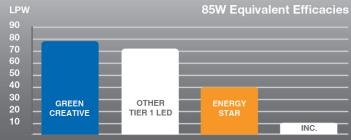
At 79 LPW, this lamp's efficacy is more than 10% higher than the Tier 1 LED BR40 85W replacement industry average and exceeds ENERGY STAR requirements by upwards of 95%. This energy-saving performance makes this lamp a smart retrofit choice for incandescent bulbs.
